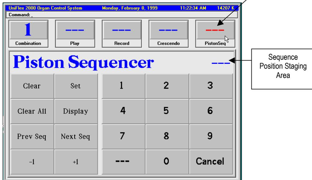
You can use the control panel to operate the piston sequencer directly if you want to try it out without installing additional hardware, however, the Piston Sequencer is designed to be controlled from CONSOLE PISTON HARDWARE.
