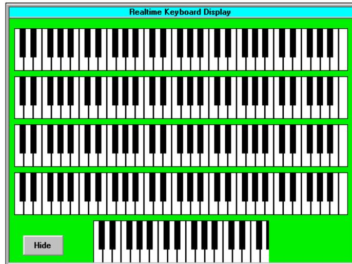
This display can be used as a diagnostic when checking out the keyboard wiring, or it can display the keying of a playback. To put away the keyboard display, touch the **Hide** button in the lower left hand corner.
