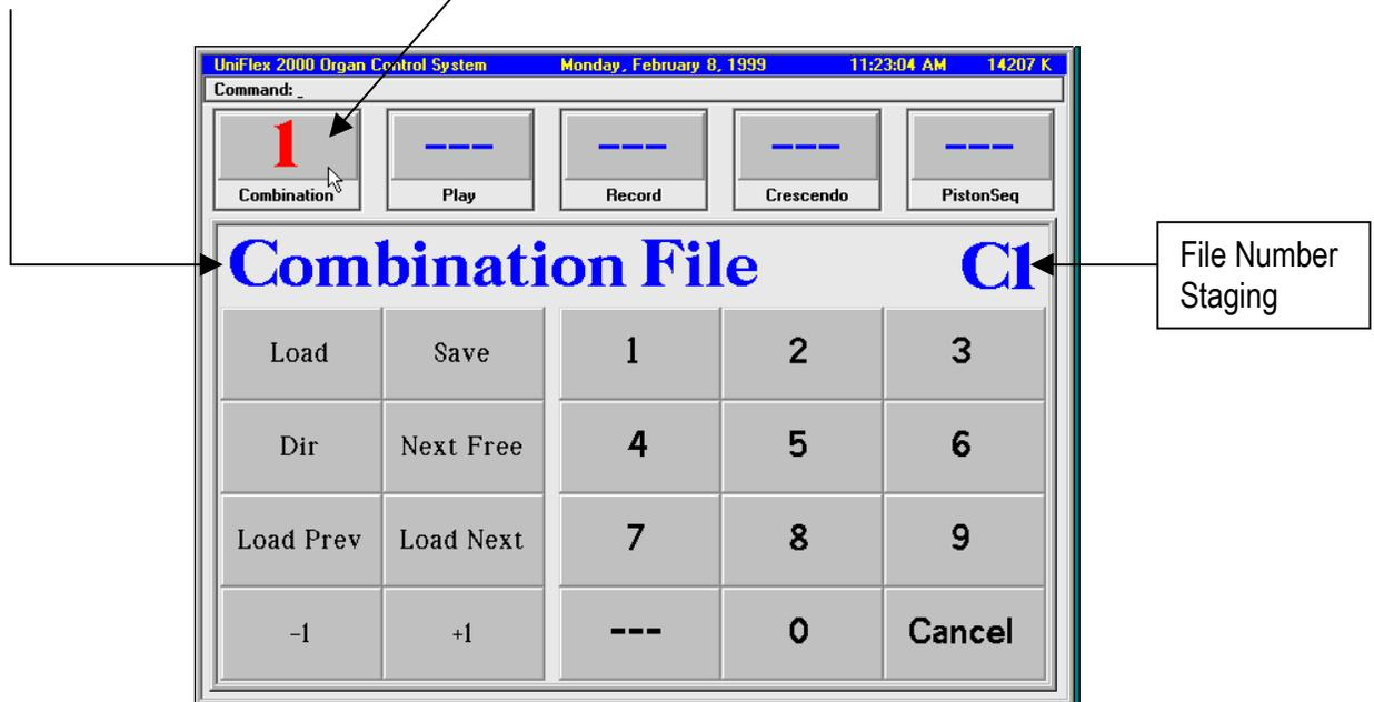
The Combination Action Control Panel will overlay the normal RUN screen and allow you to Load, and Save combination action piston files. The control panel is designed to give you just the control buttons you would need to load and save combination action files during a performance.
