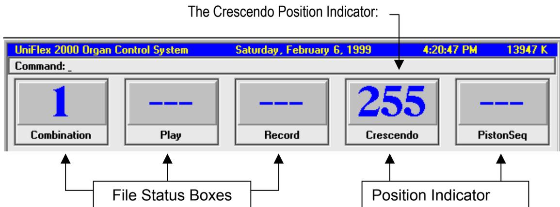
During the normal RUN-time system operation, the position of the crescendo pedal position is always indicated in the Crescendo position indicator box. The minimum and maximum values are from - - - blank (off) to 255 (full on).
