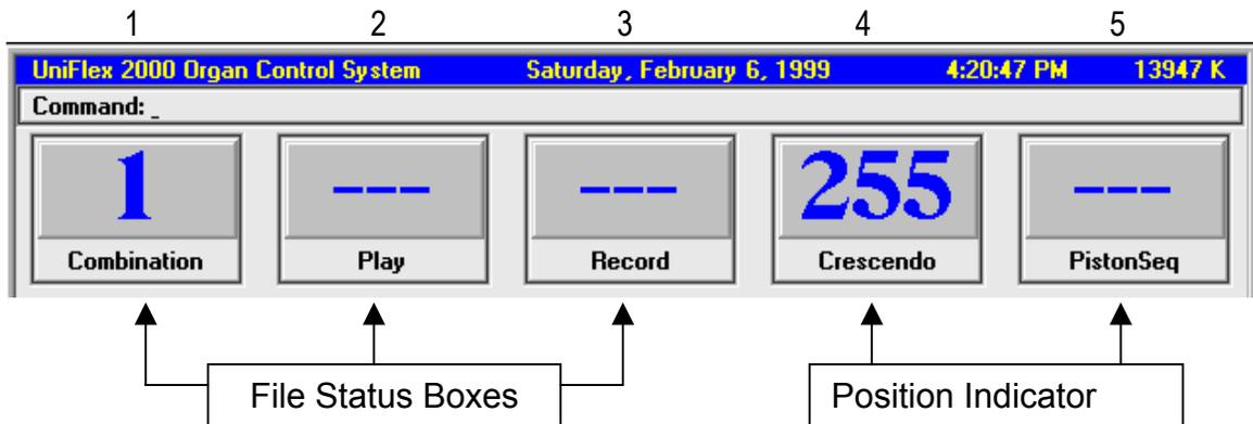
The File status and current position boxes have a dual purpose. If you are using a touch screen monitor or a mouse, touching or clicking on any of the File Status or Position Indicator Boxes, you will present you with a control panel for the specific box you have selected.
