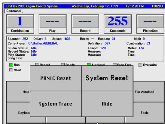
The **Tools** panel buttons are for commands you don't accidentally want to activate during normal operations or performances. The commands currently assigned to the Tools button in this software release are:
